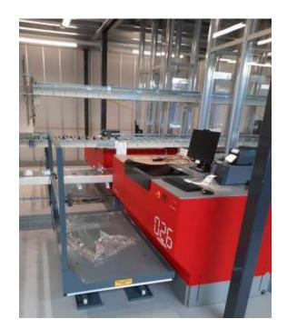
The TRANSLYFT SCB work platform is custommade for the Autostore systems. The platform makes it easy for employees of different heights to adjust the platform and work at the most ergonomic work height. It is also possible to install the work platform in a small pit.
